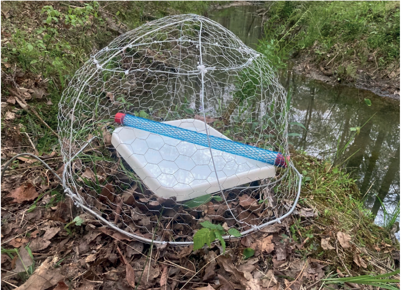
Figure 1. Size-dependent bycatch exclusion device deployed over UV light pan trap at unnamed tributary of Dick Creek in Walker County, Georgia, USA. Shown before nightfall for clarity.
